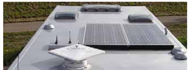
Installation Solarpanel 240W
